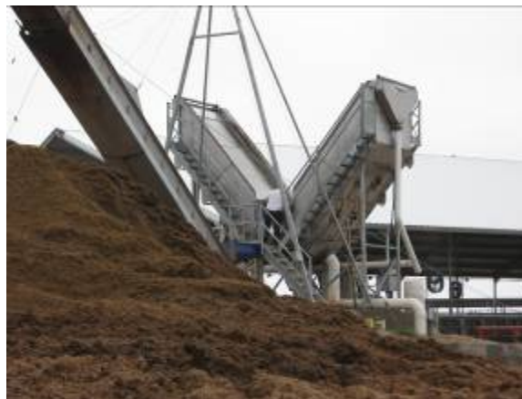
Plate 2. Dual Inclined Separation Screens
