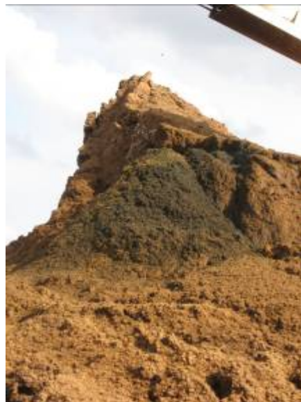
Plate 5. Coarse solids with darker portion where sludge has also been mixed in.
